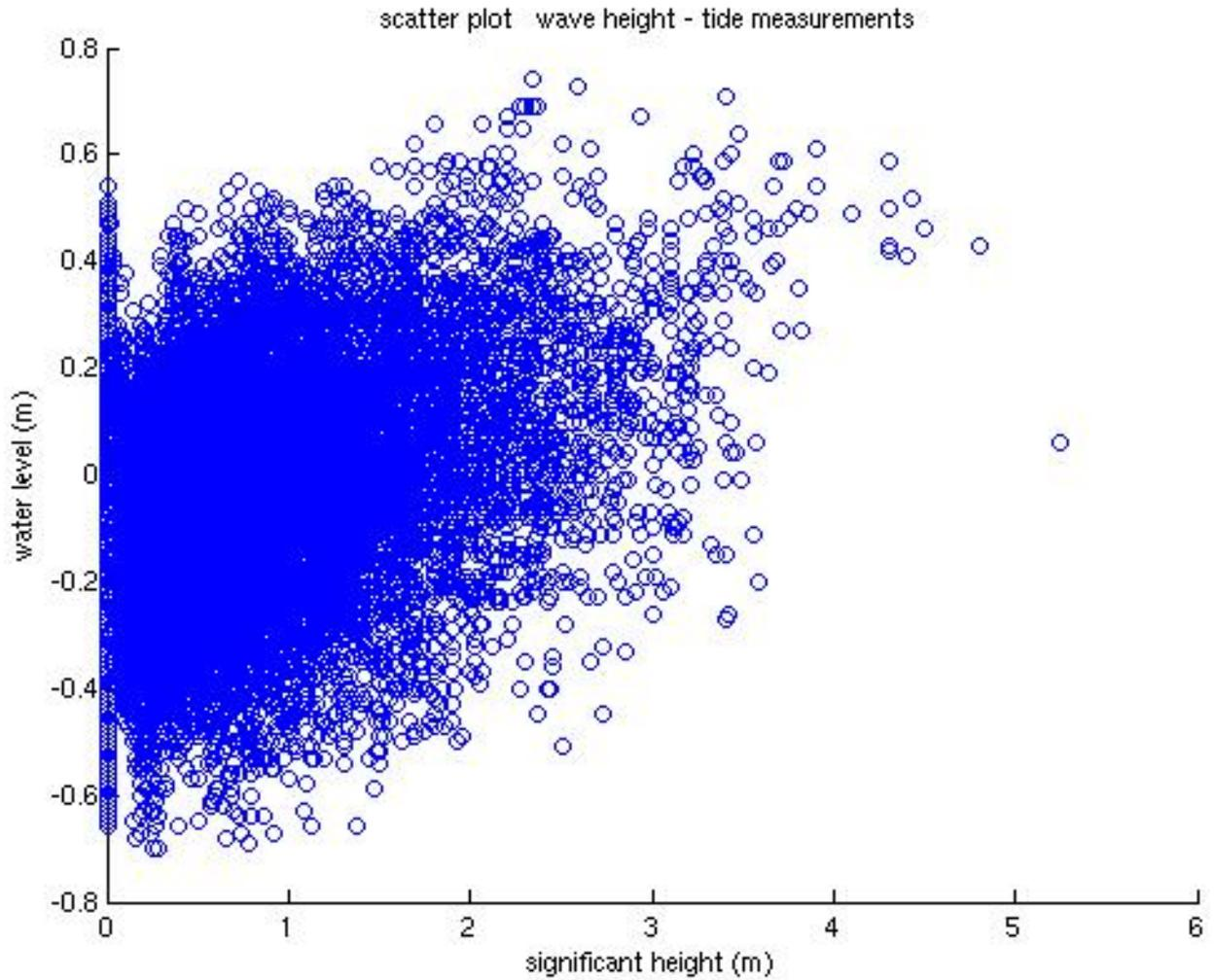
Figure 8 Scatterplot of significant wave heights and sea levels at Ancona
