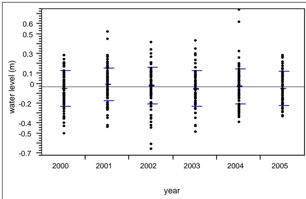
Figure 3 Oneway Analysis of Observed water level (m) by year. Only the median, 25<sup>th</sup> and 75<sup>th</sup> quantile are shown.
