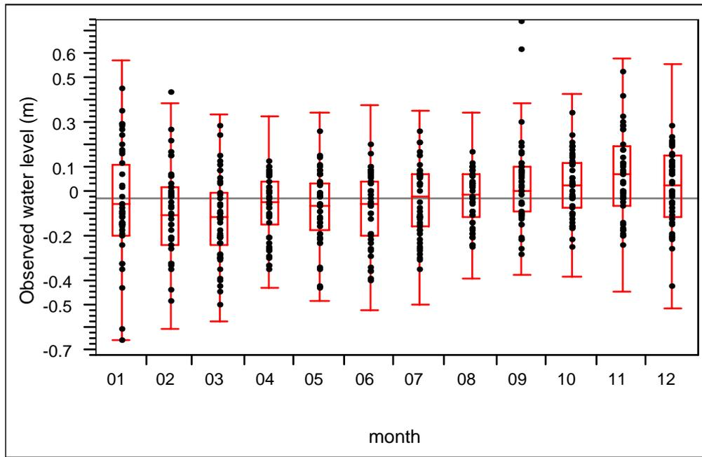
Fig. 4 Oneway Analysis of Observed water level (m) by month. In this figure is shown also the median, the 10<sup>th</sup>, 25<sup>th</sup>, 75<sup>th</sup> and 90<sup>th</sup> quantile.
