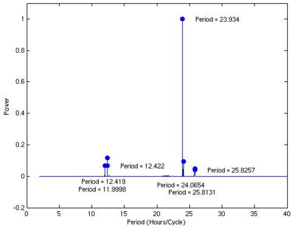
Figure 7. Tidal high frequency components at Ancona. It is worth noting the strong diurnal component, differently from the observed ones at other tide station, where the predominant component is the semidiurnal one.
